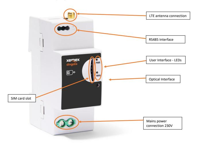
The DINgate TM gateway module is able to setup a transparent IP link between a server application and an RS485 device connected to the gateway. Data send over LTE is forwarded transparently to the RS485 interface and vice versa.
