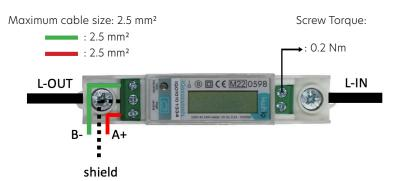
Wire the device in accordance to the Wiring Diagram. If the bare wire is visible above the terminal bridge, shorten the stripped part of the wire.
