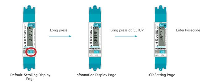
Enter the passcode in the Setting Page (factory settings: 5947). Short press to alter the blinking number. Long press at a blinking number to enter it.
